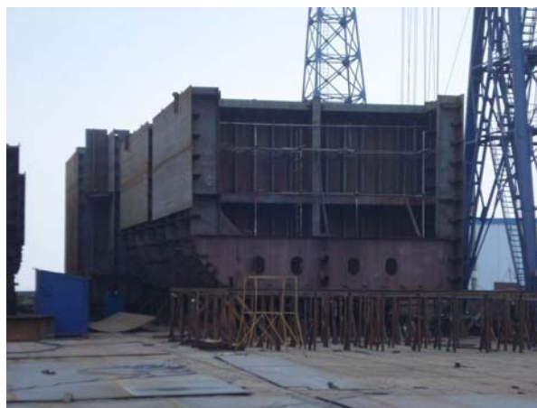
Mid ship section blocks at Nantong Yahua Shipyard
