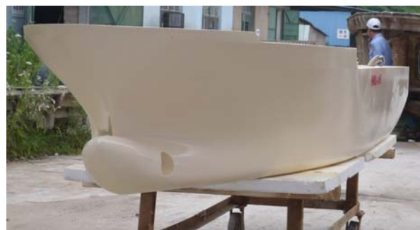
Scale model (5.2 meter length) for tank tests
